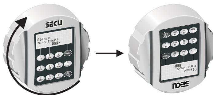
2. If the input unit is turned back to its starting position in anti-clockwise direction after the five-second ready-for-opening period, the lock will return to the blocked position and can only be unblocked after renewed clearing and re-entry of a valid code.
